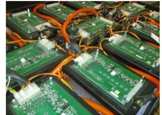
**Figure 2 Battery modules with battery management boards integrated**
