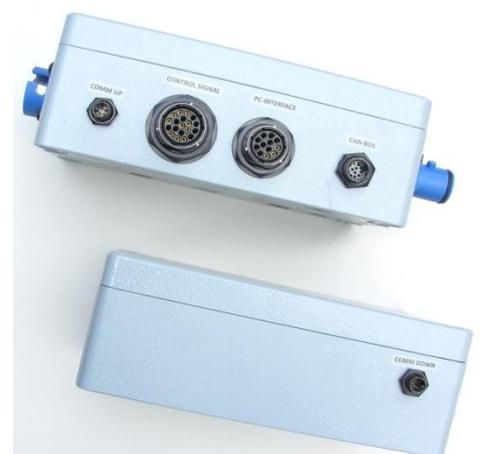
**Housed Battery Management System used in the Cyber Cab**
