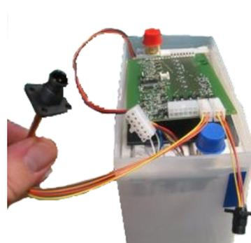
**Battery Module with Electronics shown**
