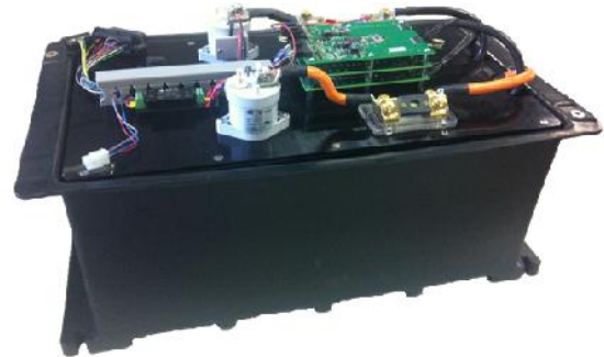
Figure 4: View of the battery pack prototype with the battery management system together with fuses and relays for redundant disconnection.
